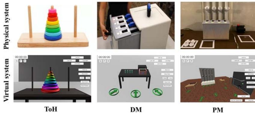
**Fig. 3.** The physical and virtual systems employed to execute the ToH, the DM and PM tasks to assess VLEARN usability and human cognitive-motor performance when performing with this simulator. ToH: Tower of Hanoi; DM: Disk drive dock maintenance; PM: Pipe maintenance.
