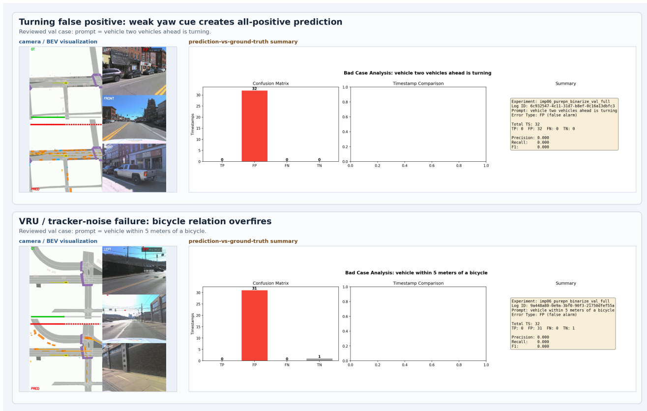
Figure 2: Reviewed validation failure modes that motivated conservative selection. Turning prompts can produce all-positive false positives when generated programs over-trust weak yaw cues. Vulnerable-road-user prompts are sensitive to tracker noise and relation thresholds, motivating track-quality diagnostics rather than global filtering.
