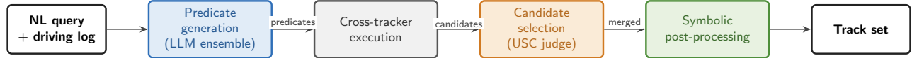
Figure 1. The Predicate architecture turns a natural-language query and a driving log into a final track set through four stages: predicate generation across an LLM ensemble, cross-tracker execution, a label-free per-frame union vote across the LLMs on the primary tracker, and a symbolic post-processing chain. Concrete LLM, tracker, and filter choices are described in §2.1–§2.4.
